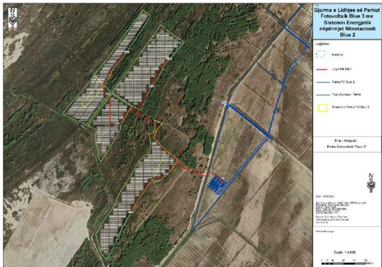
Figure 5. Blue 3 Project Layout and alignment of the grid connection corridor for the FV Blue 3 Solar Park through the Blue 2 Substation
